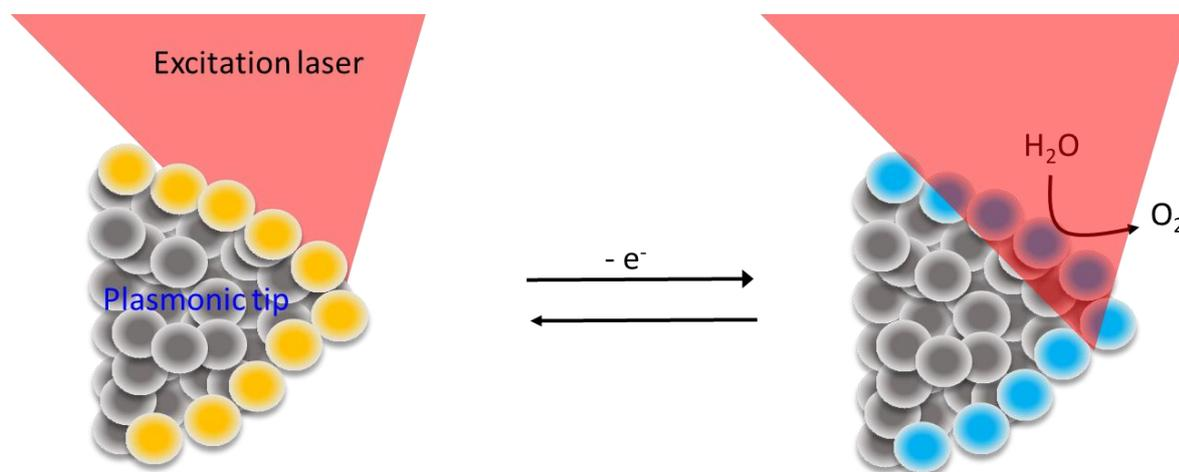
*Sketch of the EC Tip-SERS experiment. A gold or silver tip is covered with an electrocatalytic material. The tip potential can be varied to trigger an electrocatalytic reaction while the Raman spectra provide information about the reactive intermediates.*
