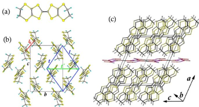
Figure 1 : Molecules BEDT-TTF (a) and their stacking along the **a** (b) and **b** (c) directions. The anion plane is shown in (c).
